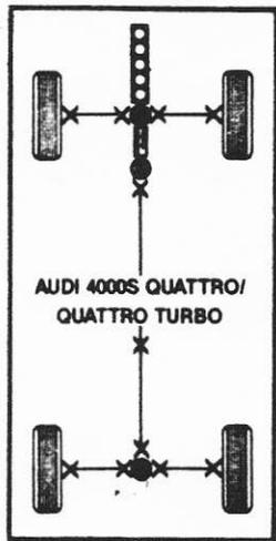
○○○○ ENGINE      ⊠ TRANSFER CASE      ● OPEN DIFFERENTIAL
